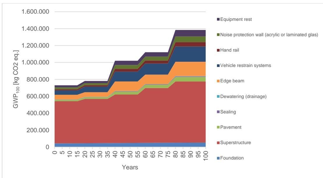
Figure 8: Time-dependent emissions over the life cycle (GWP<sub>100</sub>)
