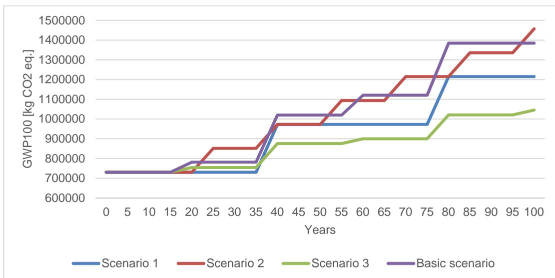
Figure 10: Time-dependent emissions ( $GWP_{100}$ ) over the life cycle for all maintenance scenarios
