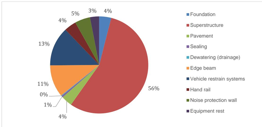
Figure 9: Contribution of the structure parts to emissions over the life cycle ( $GWP_{100}$ )
