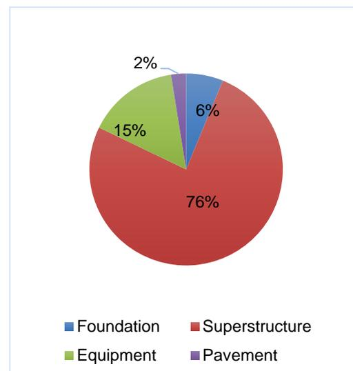
Figure 5: Contribution of the structure parts to  $GWP_{100}$  (A1-A5)
