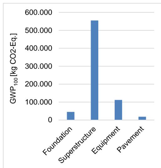
Figure 4: Results for the  $GWP_{100}$  (A1-A5) [kg CO<sub>2</sub> Eq.]
