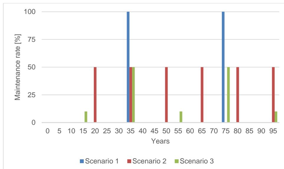
Figure 3: Time-dependent maintenance action of the simplified scenarios
