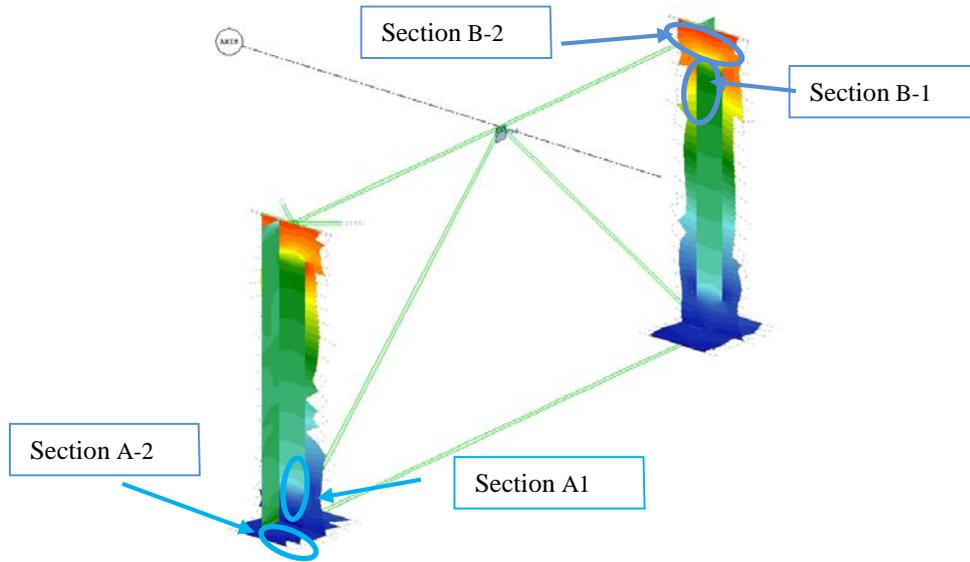
Figure 6. Sections for fatigue study
