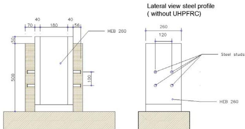
Figure 8. Example of specimen for a shear test, UHPFRC slab welded to a profile with the same dimensions as the bridge girder flange.
