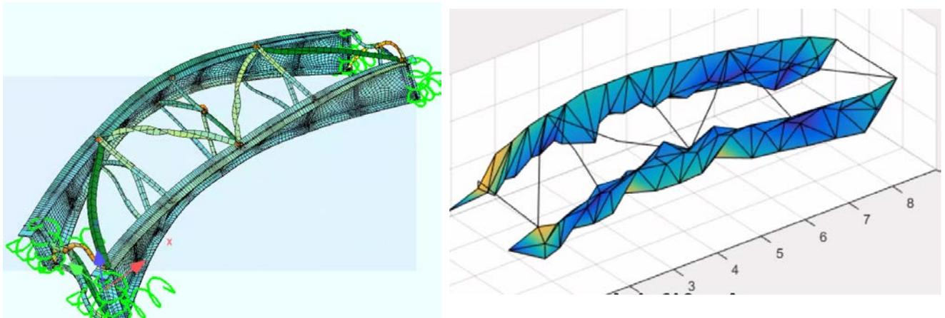
Figure 4. Mode number one, in SOFISTIK (left) and from the dynamic experiment (right).
