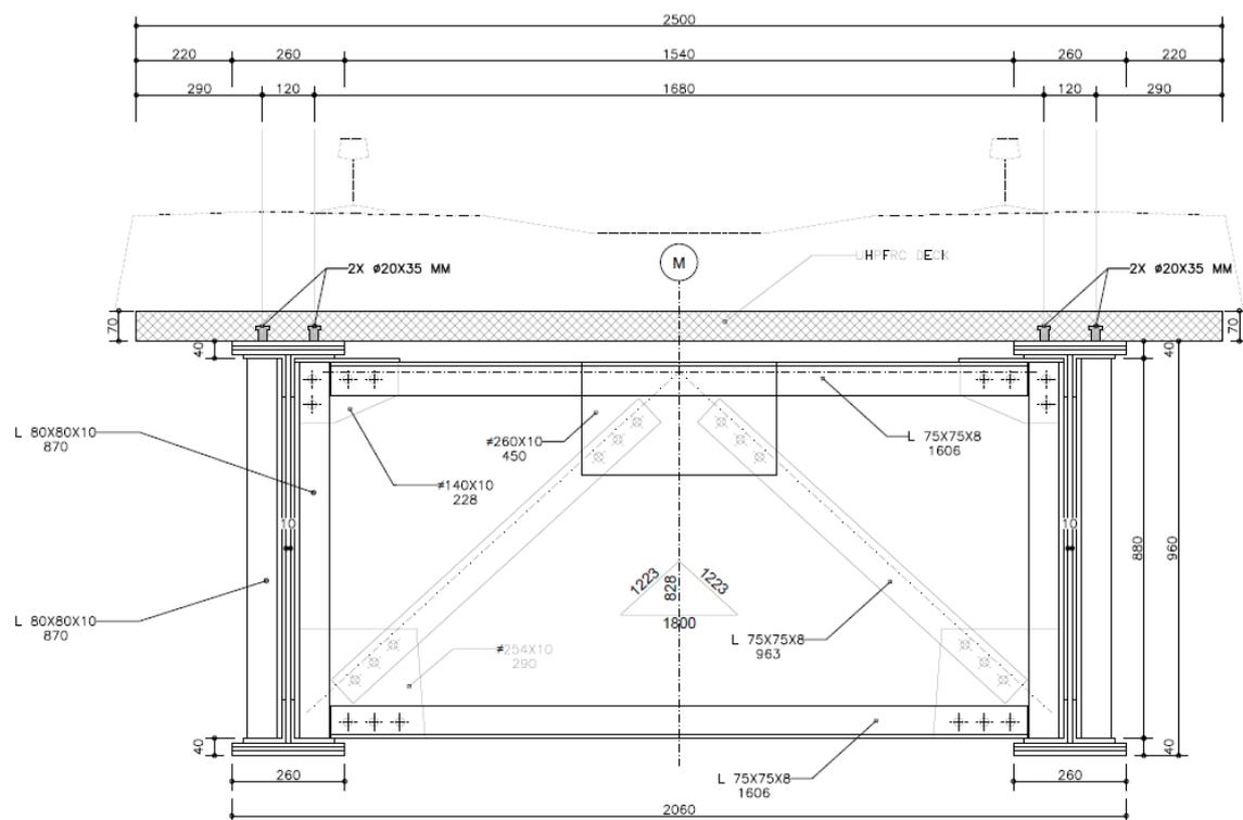
Figure 7. Typical section of the bridge after rehabilitation.
