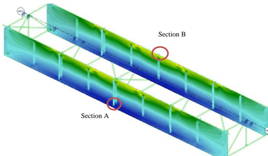
Figure 5. Most problematic sections for fatigue analysis.
