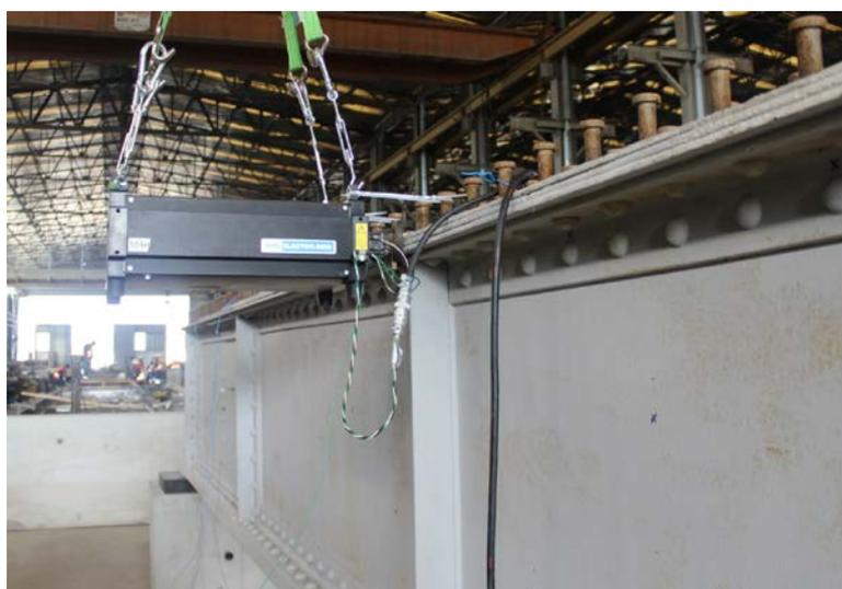
Figure 3. Shaker mounted in lateral direction for dynamic testing.
